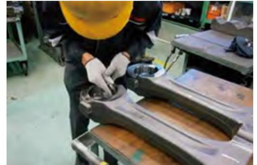
Time reduction achieved by altering and changing the tools and chamfering methods for rods
